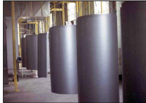
Connell Wagner's engineers were also required to inspect the quality of daily production, checking 'roundness' and dimensional accuracy of the 1100 GlennGRC™ panels produced.
